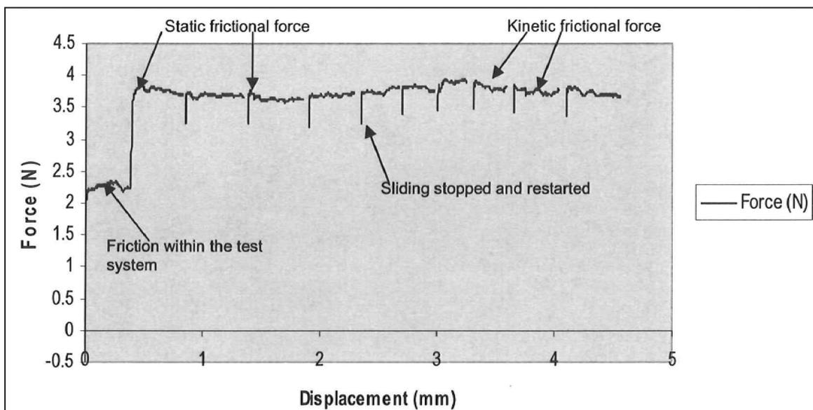
**Figure 3.** Example of the force-displacement graph pattern using the same bracket (conventional metal) over new stretches of wire. The initial rise in force represents the friction within the test system.
