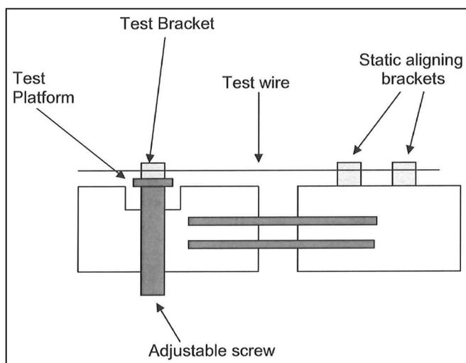
**Figure 1.** Lateral view of the specially constructed jig.
