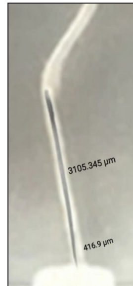
Figure 2. Fractured file segment and measurement of its length.
